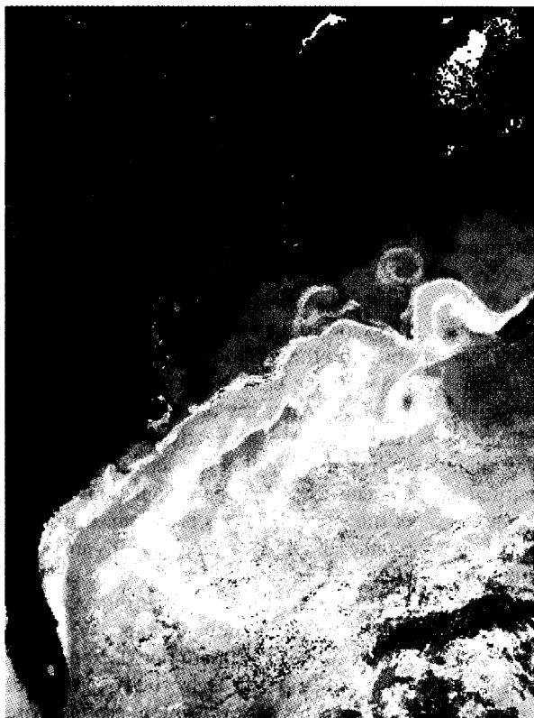
Sea surface temperature in the western North Atlantic. Orange and yellow indicate warm water; purple, blue, and green show cold water. The Gulf Stream leaves the coast at Cape Hatteras, meanders, and small eddies form. Although the eddies are constantly changing, they have an average effect on the ocean climatology. [Image courtesy of T. Lee, Massachusetts Institute of Technology; data courtesy of R. Evans, University of Miami]
