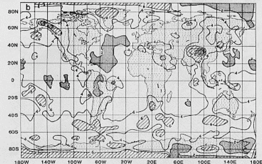
FIG. 5. The rms difference between the 6 h forecast of the 300 mb geopotential height field and the analysis for the period 5-21 January 1979. Contour interval is 20 m. a) Rms difference between the NOSAT analysis and forecast. b) Rms difference between the FGGE analysis and forecast.
