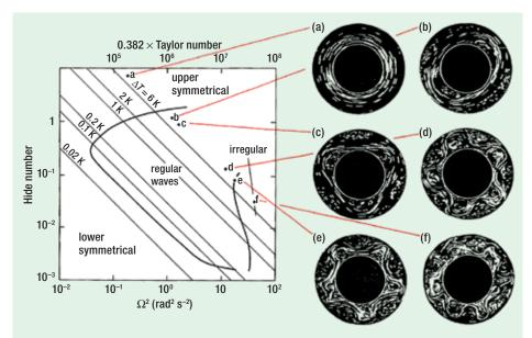
2: Flow patterns and their localization in the plane of the most important dimensionless control parameters (*H*, *T*). (Left): Experimental regime diagram, in which *T* is replaced by a stability  $\Omega^2$ . (Right): Collage of upper-level flow patterns, visualized as streak trajectories, from panel (a) to panel (f).
