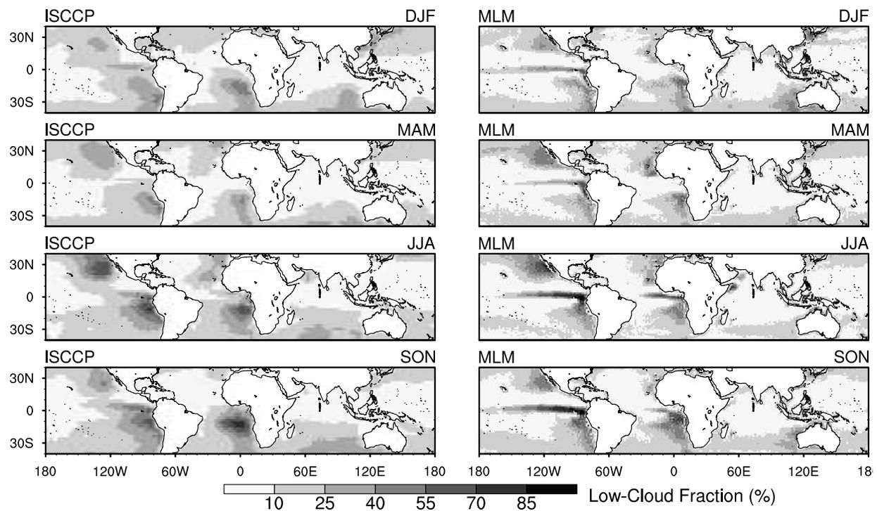
FIG. 7. Seasonal mean low-cloud fraction measured by ISCCP (left) and indicated from the mixed-layer model equilibria with daily forcing (right) over ocean averaged in 12 years (1990-2001).
